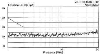
Figure 4 – MIL-STD-461C Two VPT15-2800S With VPTF3-28 EMI Filter
