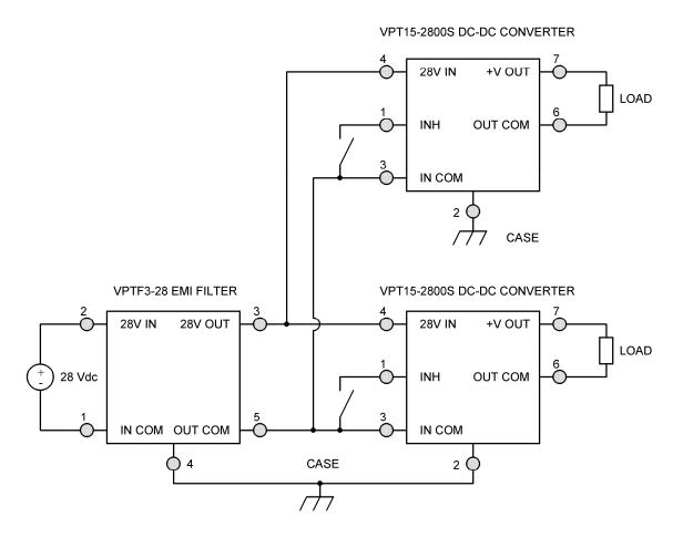
Figure 3 (Shown with multiple VPT Series DC-DC Converters)
