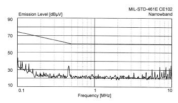
Figure 5 – MIL-STD-461D/E Two VPT15-2800S With VPTF3-28 EMI Filter
