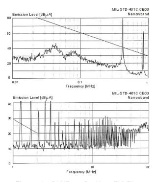
Figure 13 - DVHF2800D without EMI Filter
