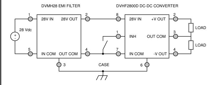
Figure 6 – Converter with EMI Filter
