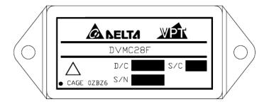
Figure 1 – DVMC28 / DVMC28F EMI Filter (Exact marking may differ from that shown)
