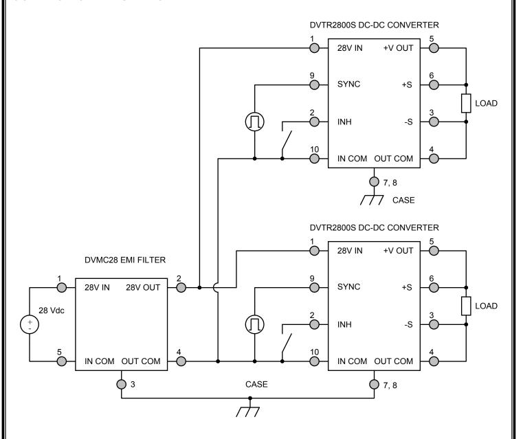
Figure 4 – DVMC28 EMI Filter Hookup with Two Converters
