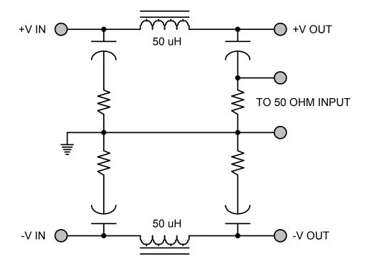
Figure 6 – MIL-STD-461D Measurement Method (LISN)
