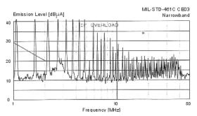
Figure 7 – MIL-STD-461C DVTR2800D Without EMI Filter
