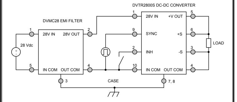
Figure 3 – DVMC28 EMI Filter Hookup with Single Converter
