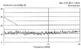
Figure 8 – MIL-STD-461C DVTR2800D With DVMC28 EMI Filter
