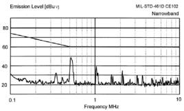
Figure 10 – MIL-STD-461D DVTR2800S With DVMC28 EMI Filter
