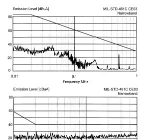
Figure 9 – MIL-STD-461C Two DVTR2800S's With DVMC28 EMI Filter
