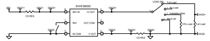
Figure 15 – Radiation exposure circuit (TID)
