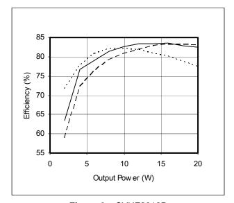
Figure 8 – SVHF2812D Efficiency (%) vs. Output Power (W)
