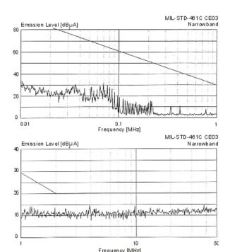
Figure 14 - SVHF2800D with EMI Filter
