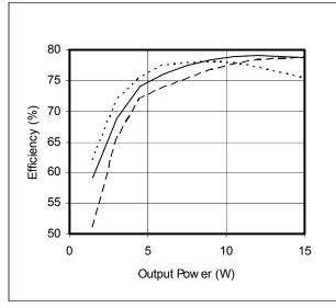
Figure 7 – SVHF2805D Efficiency (%) vs. Output Power (W)
