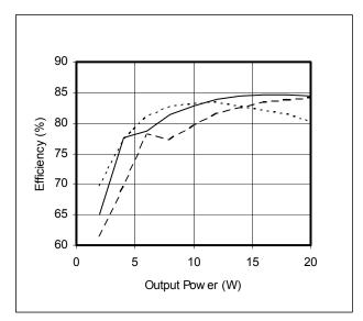
Figure 9 – SVHF2815D Efficiency (%) vs. Output Power (W)
