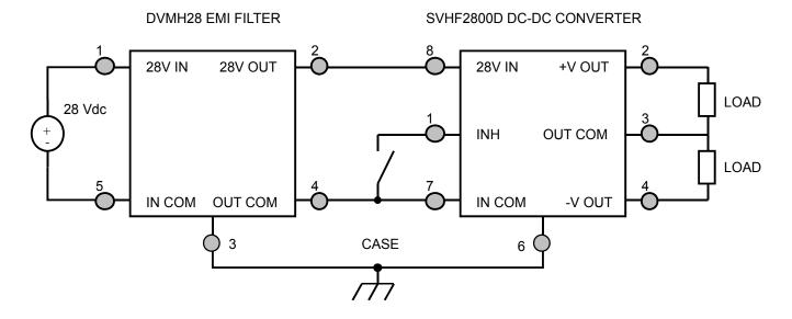
Figure 6 – Converter with EMI Filter
