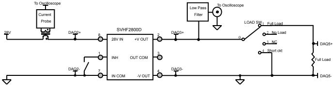
Figure 16 – Radiation exposure circuit (SEE)
