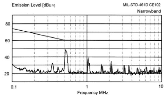
**Figure 9 – MIL-STD-461C Two DVTR2800S's With DVMC28 EMI Filter**
