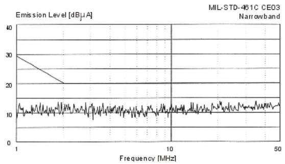
**Figure 7 – MIL-STD-461C DVTR2800D Without EMI Filter**
