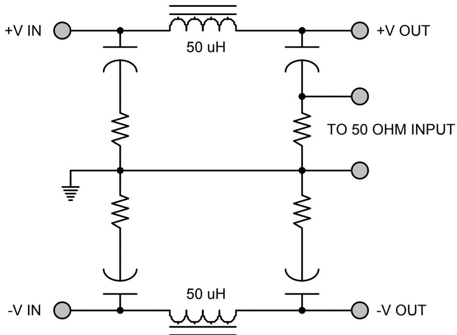
Figure 6 – MIL-STD-461D Measurement Method (LISN)
