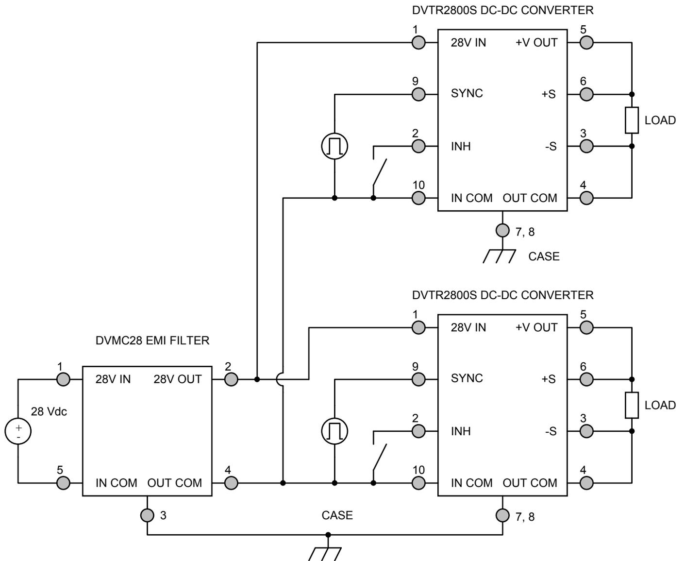
Figure 4 – DVMC28 EMI Filter Hookup with Two Converters
