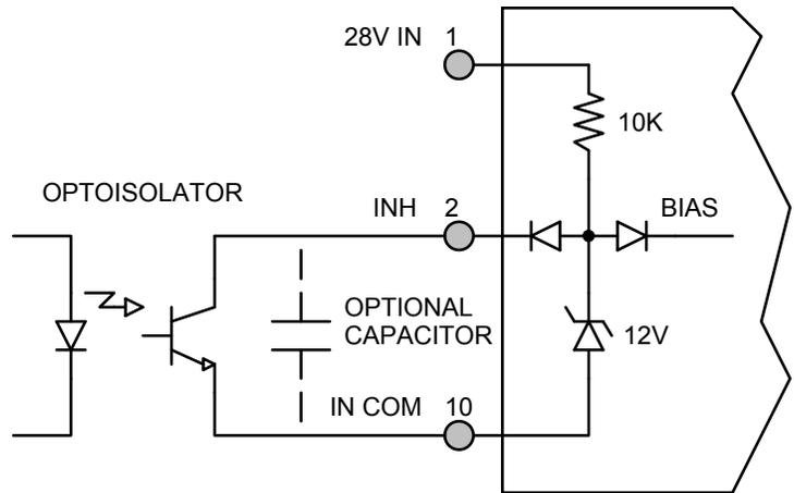
**Figure 5** – Isolated Inhibit Drive
