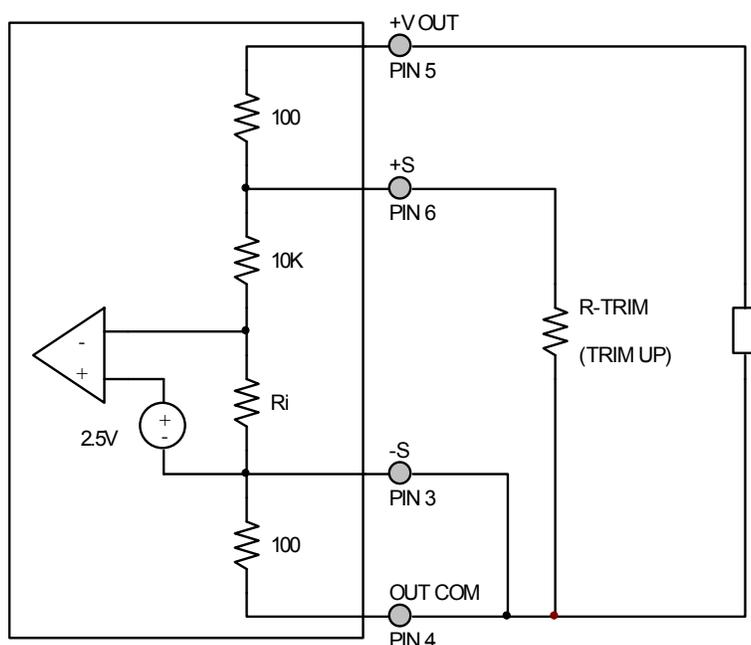
The output voltage can be trimmed up by connecting a resistor between the +S pin (PIN 6) and the OUT COM pin (PIN 4). The maximum trim range is +10%. The appropriate resistor values versus the output voltage are given in the trim table below. The -S pin should be connected to the OUT COM pin.
