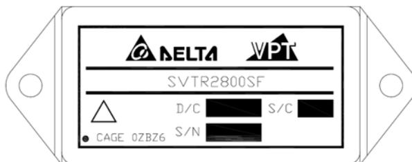
Figure 1 – SVTR2800S / SVTR2800SF DC-DC Converter (Exact marking may differ from that shown)
