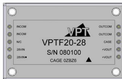
Figure 1 – VPTF20-28 EMI Filter (Not To Scale)
