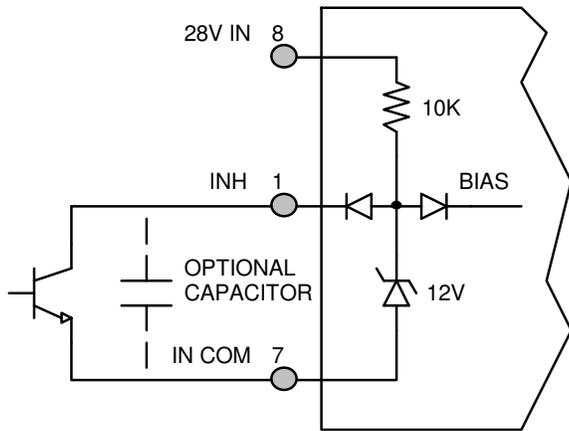
**Figure 4** – Internal Inhibit Circuit and Recommended Drive
