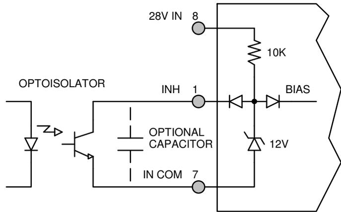
**Figure 5** – Isolated Inhibit Drive
