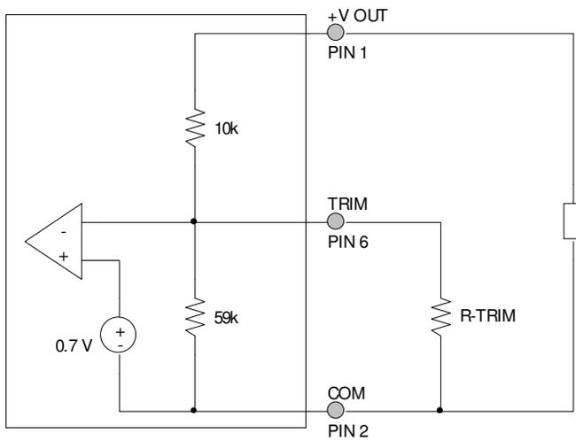
The output voltage is set with an external resistor connected from the TRIM pin to GND pin. This resistor must have a tolerance of 1% or less to achieve an accurate output voltage.
